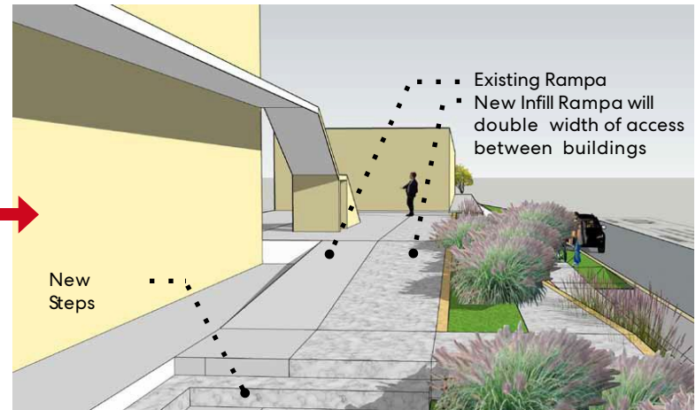
View of proposed filling of existing rampa to widen connection between buildings
